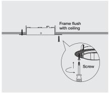
2. Secure trimless kit onto ceiling with screws.
